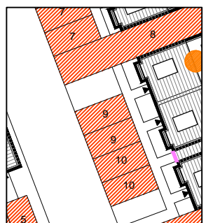
Parking spaces to be block paved
